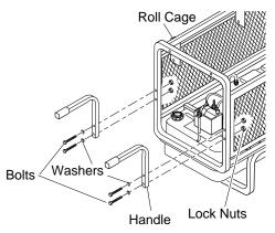
Figure 8 - Attaching Handles to Roll Cage
